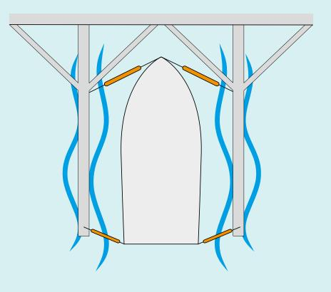
Most rubber compensators on the market must be threaded when fitted to the line. However, some products – such as Unimer's U-Cleat Mooring Compensator and Smart Snubber – do not require a free end, giving you plenty of options over a conventional compensator. The compensator can easily be repositioned after fitting, transferred to another line, or attached to a line with eye splices or thimbles on both ends. Smart Snubber can even be connected to already fastened lines.
